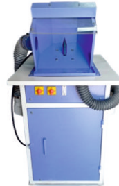
LAPPING STATION WITH DUST COLLECTOR
