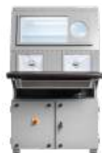
FILLING TABLE WITH DUST COLLECTOR
